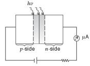
the junction field and made to flow across the junction, creating reverse current across the junction. The value of reverse saturation current increases with increase in the intensity of incident light. It is found that the reverse saturation current through the photodiode varies almost linearly with the light flux.
